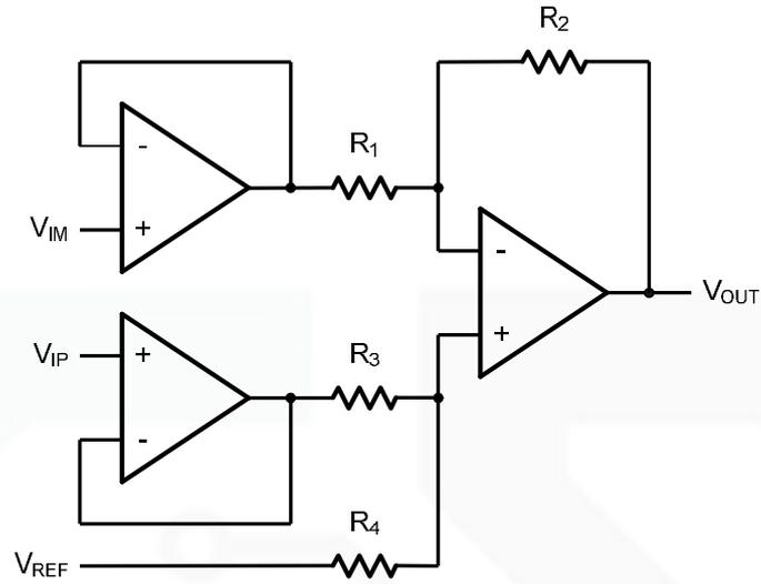
Figure 6. Instrument Amplifier
