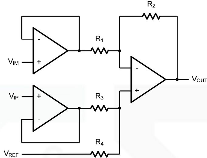
Figure 6. Instrument Amplifier
