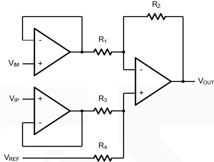
Figure 6. Instrument Amplifier
