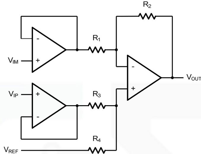
Figure 6. Instrument Amplifier
