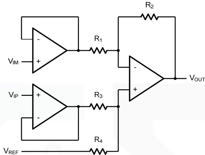
Figure 6. Instrument Amplifier
