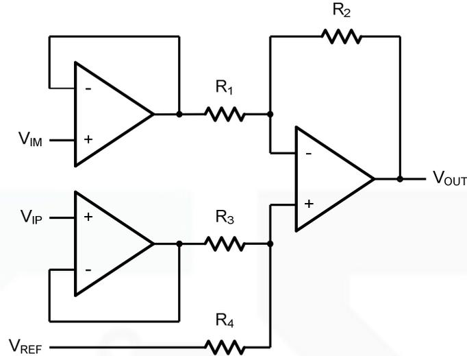
Figure 6. Instrument Amplifier
