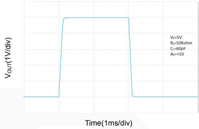
Small Signal Inverting Pulse Response
