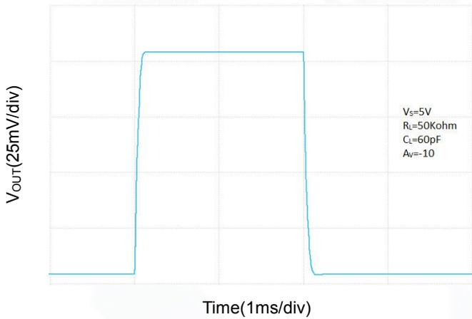
Small Signal Non-Inverting Pulse Response
