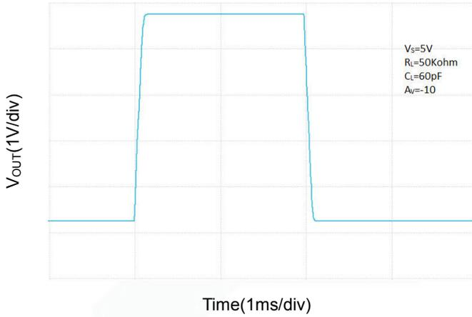
Large Signal Non-Inverting Pulse Response
