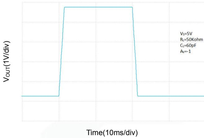
Large Signal Non-Inverting Pulse Response
