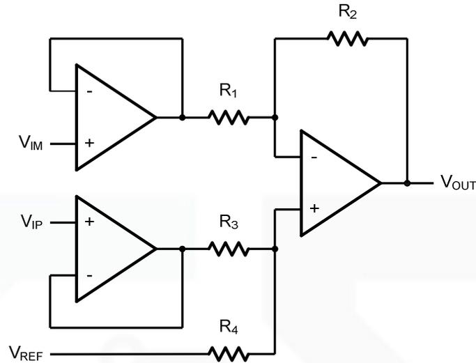
Figure 6. Instrument Amplifier
